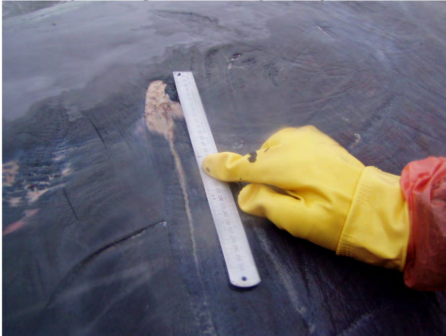
Figure 7: Rope marks showing braiding with scale
